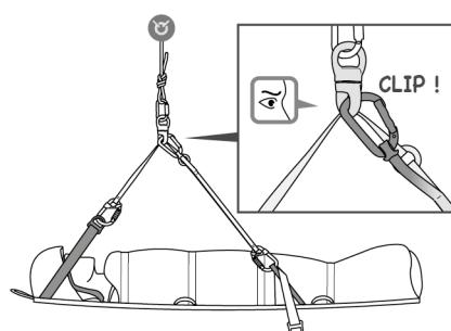
10b. Changing from horizontal position to inclined position
