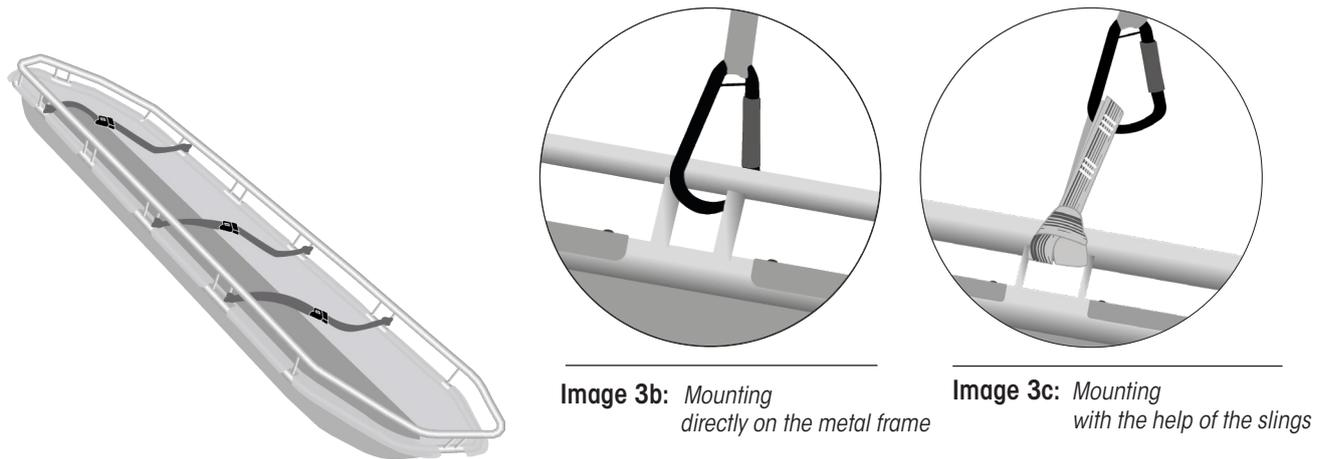
**Image 3a:** Mounting the patient restraint belts in the SAN-0087-1-M
