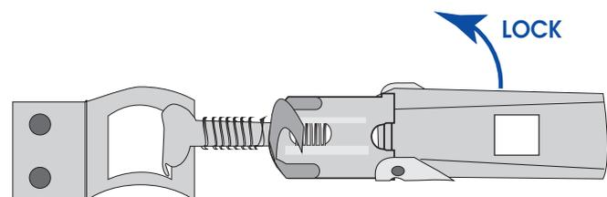
**Image 5:** Locking of the external quick-locking devices
