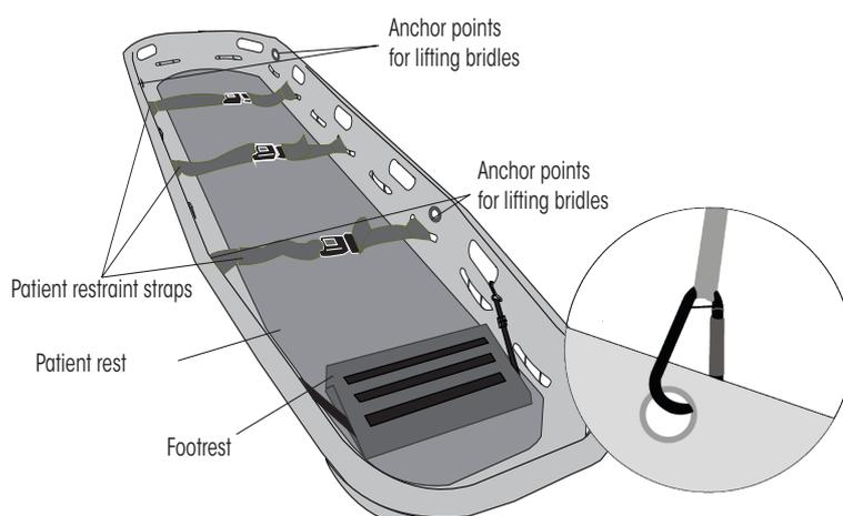
Image 1: Components of basket stretcher and anchor points
