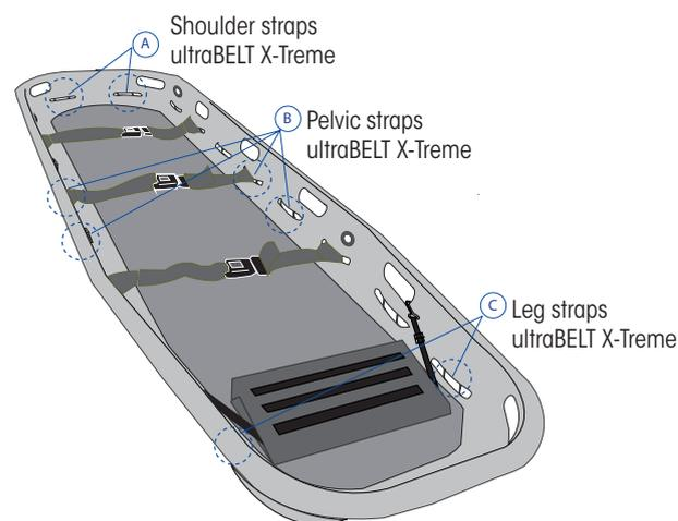
Image 7: Attaching the ultraBELT X-TREME strap system
