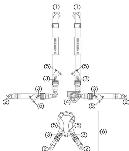
Image 6: Parts of the strap system ultraBELT X-TREME
