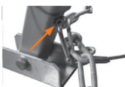
Using a carabiner, attach the eyelet of the steel rope to the eye bolt of one of the support legs. (Image 1 shows the installed chain end from assembly point 4, in addition to the installation of the steel rope eyelet.)
