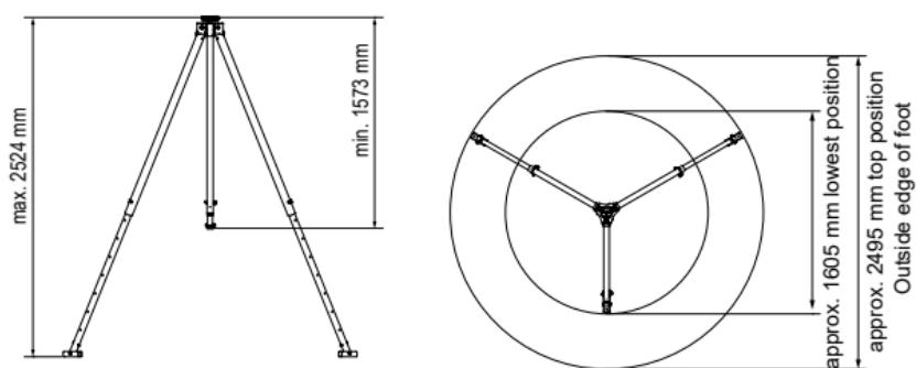
Make sure there is a level, non-slip surface so that stability is guaranteed and, in individual cases, evaluated within the scope of a thorough risk assessment. The support surface must be able to take a vertical load of at least 5kN per leg (15 kN overall including reserve).
