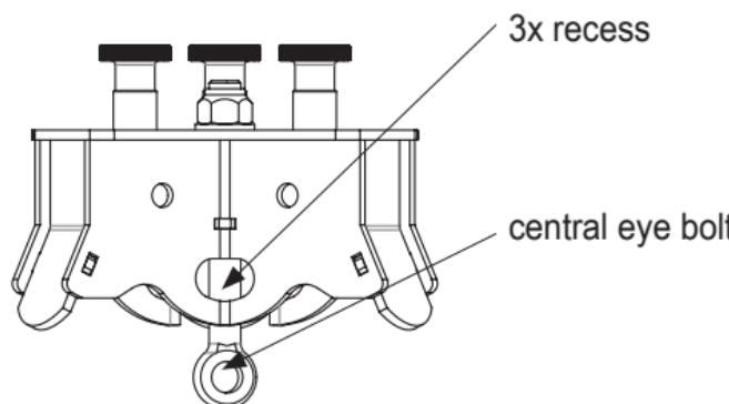
The fall arrest system for which the TRIBOC is being used as an anchor point, has to be equipped with means that restrict to 6kN dynamic forces arising during a fall. If the TRIBOC has been equipped with a load wind, tools and machine parts can also be lowered with it. The maximum permissible load is:
