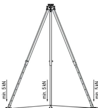
Depending on the construction situation, attention should be paid to individual fall protection even during set-up. The working area (effective direction of a fall) lies within the triangle created by the three legs and the chain. Pulling over the tripod or swinging based on the ascent or descent not being vertical to the anchor point (direction of fall, in the worst case) must be prevented under all circumstances.
