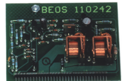
80.01.63 On-board mains voltage identification system
