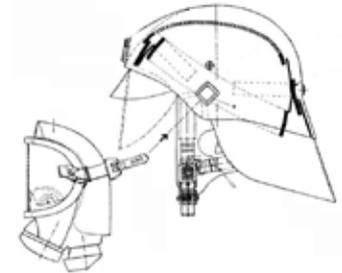
The mask can be removed again by keeping the outer pushbuttons pressed and, at the same time, pulling the mask backwards slightly with the help of the laterally attached mask straps (locking function).
