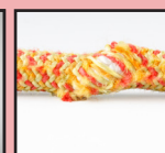
Serious sheath damage
