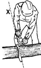
When sawing, the left arm should be almost fully extended. Guide the machine so that body parts are outside the imaginary "X" line formed by the guide rail and its extension.
