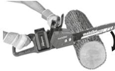
Place the pronged stop (5) of the chainsaw against the wood before starting the machine by holding it on the bow handle (7) and pulling up the switch handle (14).
