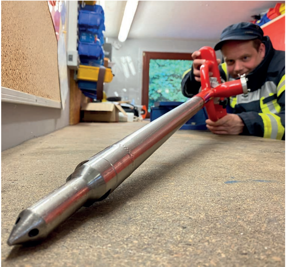
I Figure 17 Visual inspection – E-extinguishing lance® for wear
