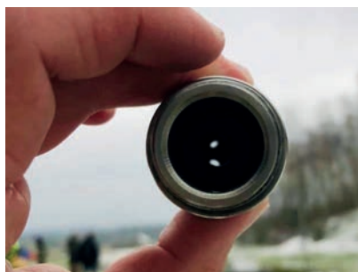
I Figure 16 Visual inspection – checking whether the E-extinguishing lance ® tip is blocked
