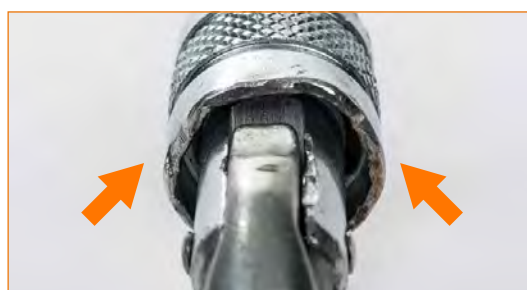
Connector with heavily damaged screw gate.
