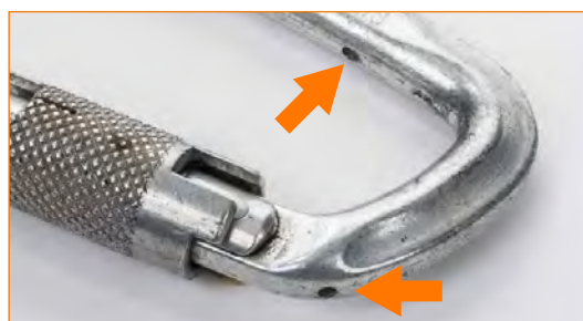
Connector with missing bar.
